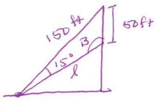
Two cables are attached to a vertical Pole on the ground as shown. Find the length of the shorter cable,  $l$ .
